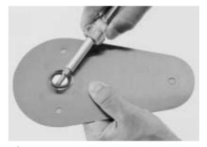
**6** Using a screwdriver, pry out the shaft seal, then throw the shaft seal away.
